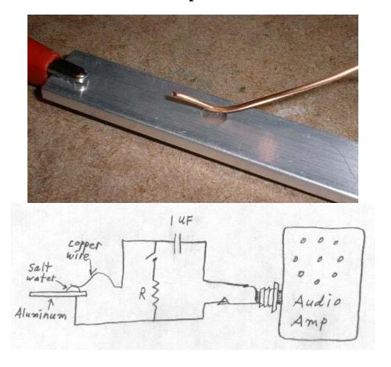
When the aluminum and contact wire above are connected to an audio amplifier, very strange and interesting sounds can be heard. This cell also produces a small voltage and there is generally more activity when R (100k to 1meg) is in the circuit drawing some current.
